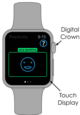
Figure 1: The Apple Watch UI: the Digital Crown wheel is used for scrolling through answer options; the touch display is used for swiping gestures and clicking the submit button.
